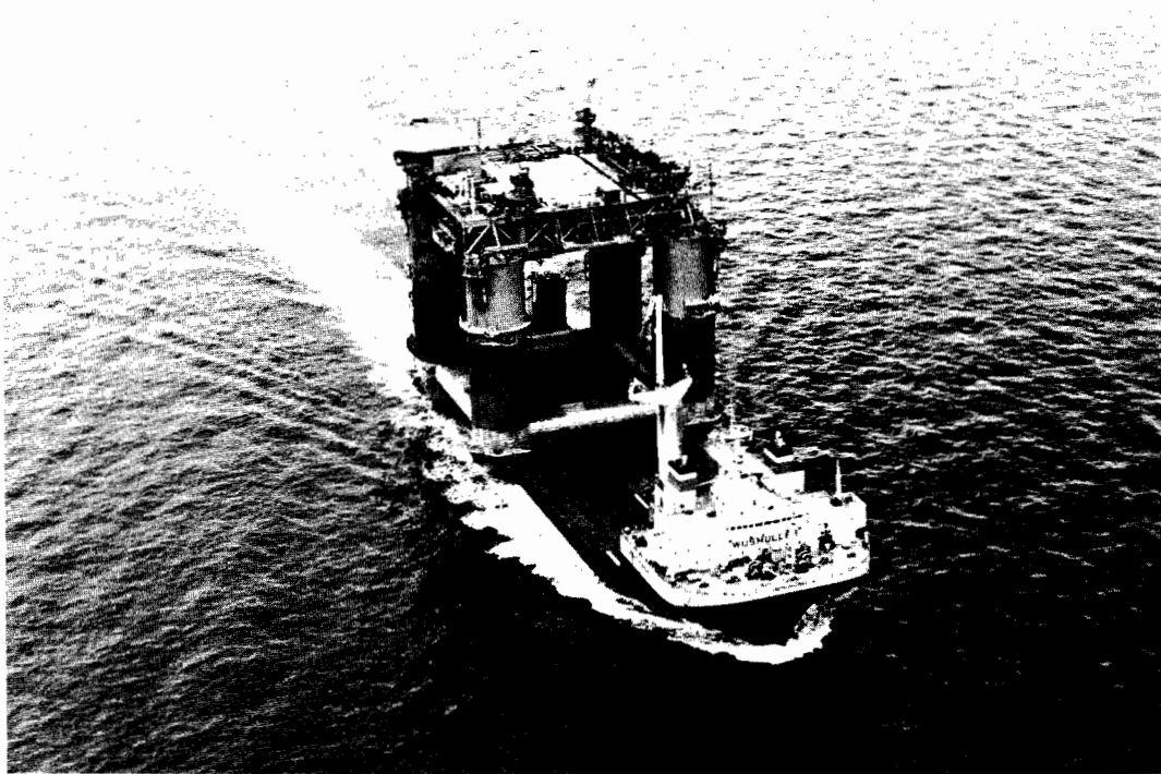
Fig. 13 - TLWP in transit onboard the Heavy-Lift ship.
