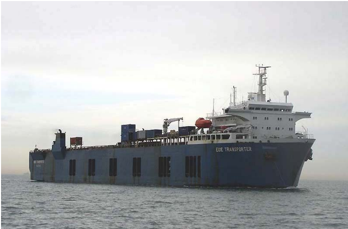
Figure 15 The 11,306 dwt dock ship Eide Transporter [11]
