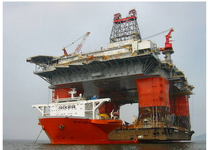
Figure 1 Jumboised Blue Marlin transporting the 59,500 t heavy Thunder Horse PDQ platform [1]
