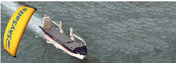
Figure 20 Beluga SkySails outfitted with a SkySails system [14]
