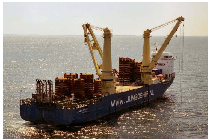
Figure 18 Jumbo Javelin installing a suction pile offshore [4]
