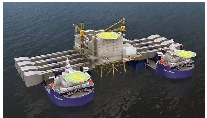
Figure 7 Twin Marine Lifters lifting a topside structure [6]
