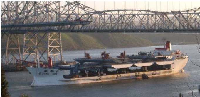
Figure 2 Zhen Hua 4 loaded with bridge sections
