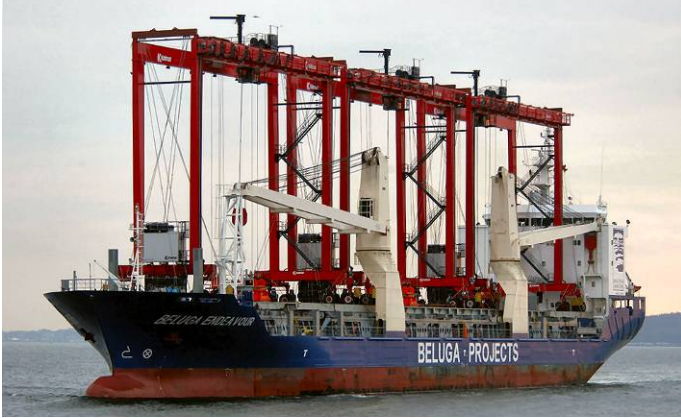
Figure 19 Beluga Endeavour with 3 RTGs on deck [13]
