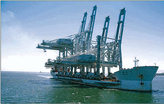
Figure 22 Zhen Hua 7 with 4 container cranes for Long Beach [19]
